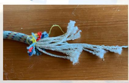
Cutting the 'sheath' (the outside bit) we can reveal 14 internal 'cores' (the white bit).
